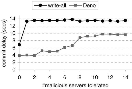
Fig. 10. Commit delay versus degree of tolerance (N = 15, TR = 0.01, SP = 2).
