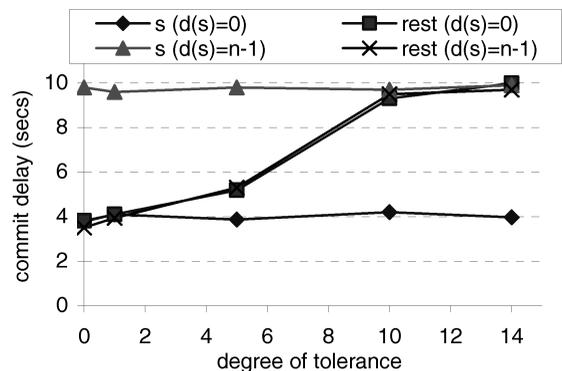
Fig. 12. Commit delays versus degree of tolerance (N = 15, TR = 0.01, SP = 2).
